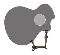
The support should now be attached to the instrument. To ensure instrument safety, a soft cloth may be placed between the support and instrument during the placement process.
